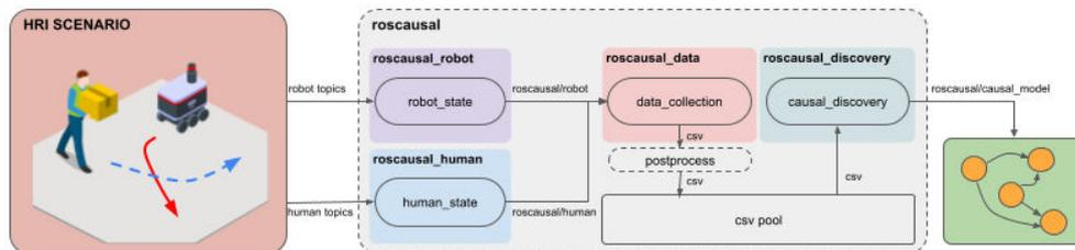
**Figure 10:** ROS-Causal pipeline: (i) data extraction from HRI scenarios; (ii) collection and post-processing of data to derive a high-level representation of the scenario; (iii) causal discovery conducted on the data, with the resulting causal model published on a dedicated ROS topic.
