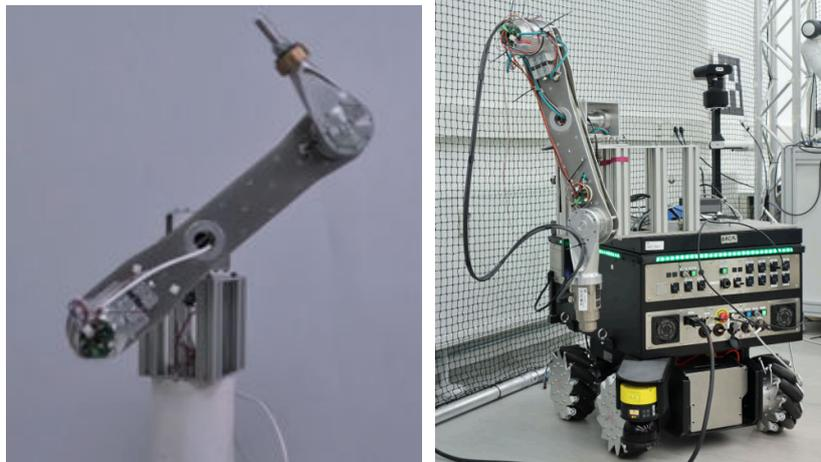
**Figure 6:** Snapshot of the developed 3-DoFs elastic arm (left) and its integration on the second mobile platform (right).
