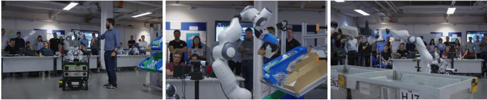
**Figure 4:** Impressions from the full scenario demonstration. DARKO robot approaching the shelf (left), a successful grasp of an item from a bin (middle), delivery and throw of the item into the target tray (right)
