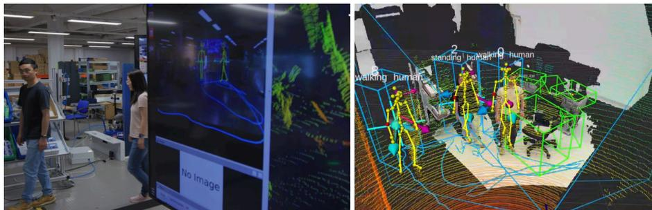
**Figure 8:** Human and object perception. The left subfigure shows impressions from the demo at KI.Fabrik during the stakeholder meeting. The right subfigure depicts example output of the DARKO 3D perception stack with tracked humans and their articulated poses (skeletons), detected objects and recognized activities.
