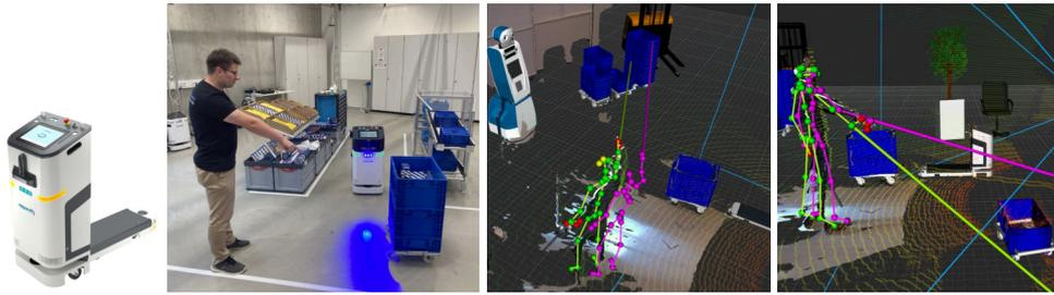
**Figure 9:** Intuitive robot control via pointing gestures demonstrated in Bosch robotics lab. From left to right: the ACTIVE Shuttle – an autonomous robot used to transport items e.g. in shopfloors of manufacturing plants; an example of pointing gesture; visualization of 3D pose estimation results by several methods from DARKO human perception stack, and the resulting semantic map with inferred pointing directions.
