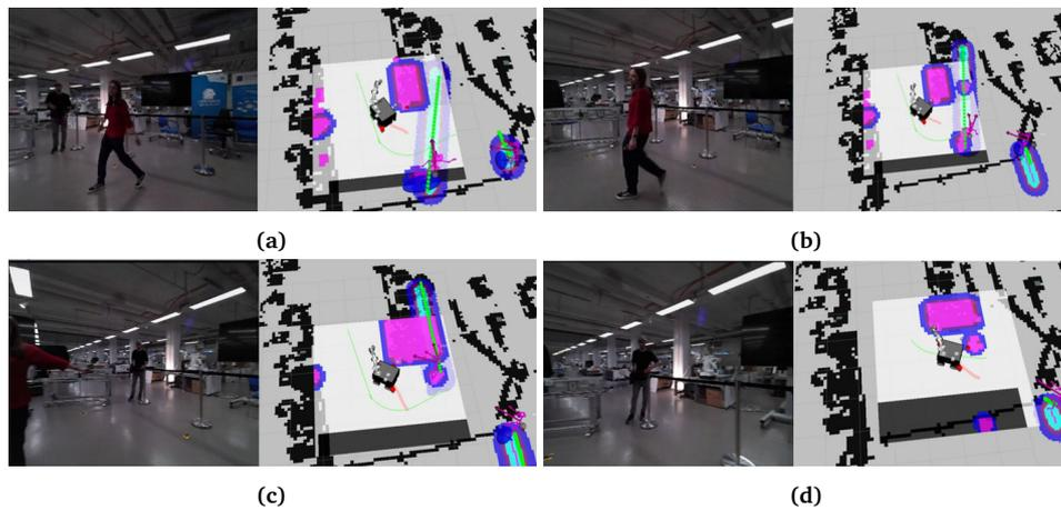
**Figure 12:** Rviz visualization and onboard camera image, while the robot moves in the KI Fabrik. The risk map is centered on the robot and includes detected objects, and static known risky areas (near the retractable belt stanchions).
